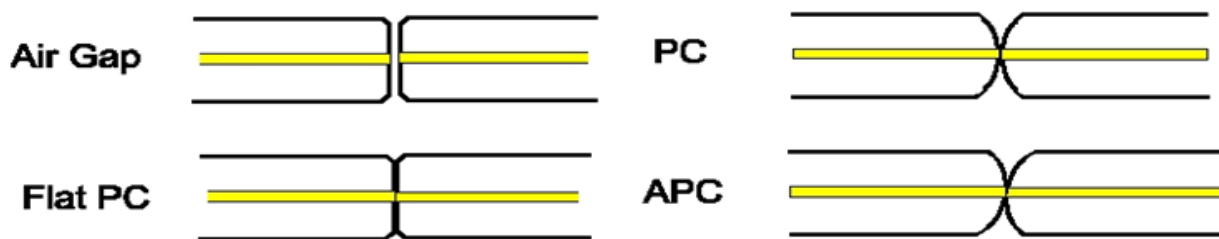
Illustration 7. Connector ferrule shape and polishes
