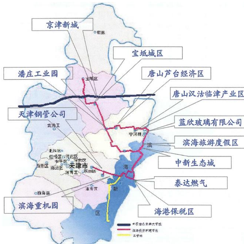
Illustration 1. Gas supply and main distribution network running within Tianjin
