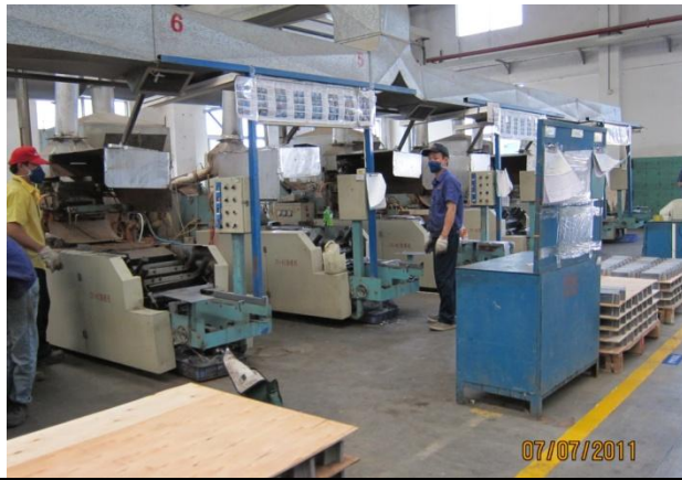
Photo set 2. Production lines of grids and batteries
